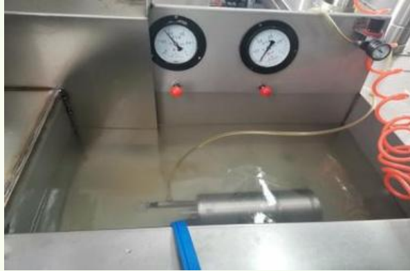
Motor sealing test
