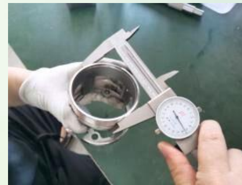
OUTSIDE DIAMETER INSPECTION
