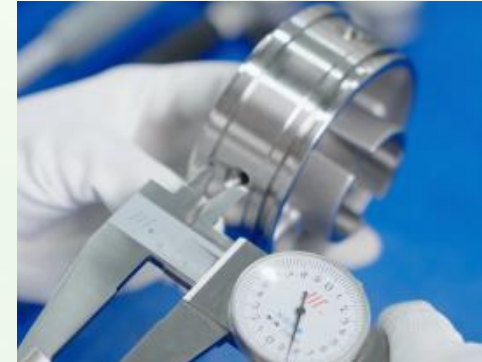
INNER DIAMETER INSPECTION
